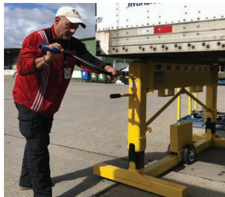
In Germany, Germesheim DC's Rene Wieland sets up a jack on a parked trailer to keep his co-workers safe while loading.
