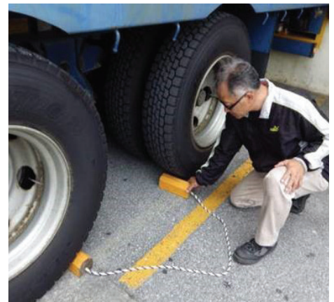
Okinawa DC's Shosei Okuhama places blocks against a truck's tires to prevent the vehicle from possibly rolling off.
