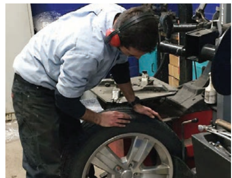
Jason Cartee at Germany’s Hohenfels Car Care Center protects his hearing while working with a loud air-pressure gun and tire-balancing machine.
